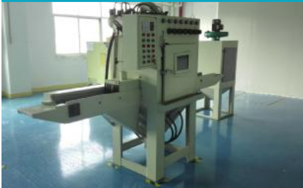
Automatic Sand Blasting
